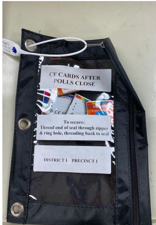
Figure 17 – Sealing the Black Zipper Pouch for CF Cards
